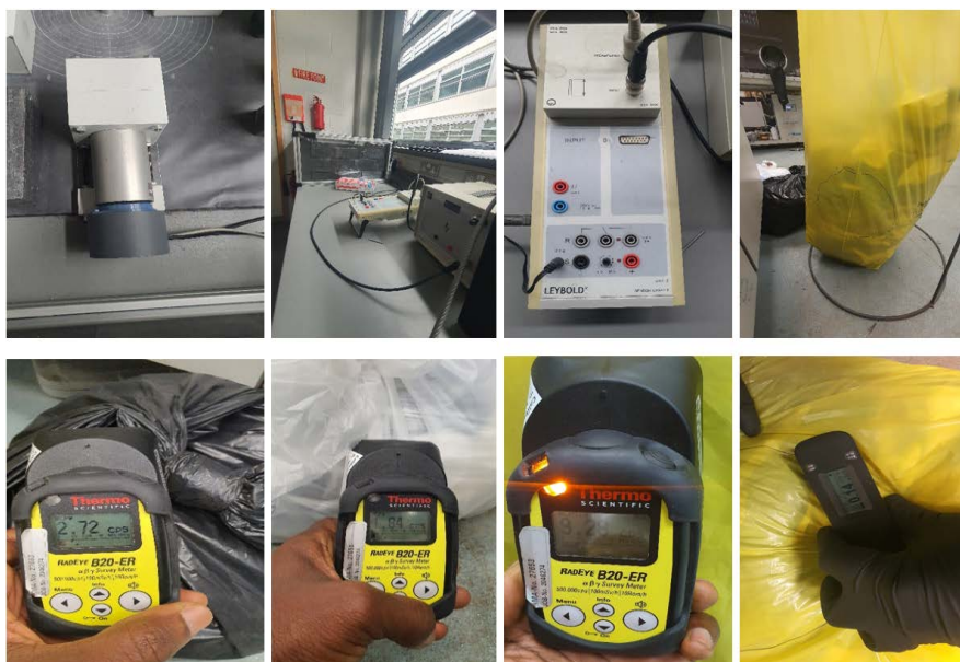
Figure 1. Display of instrumental setup for radiation dose measurements.
