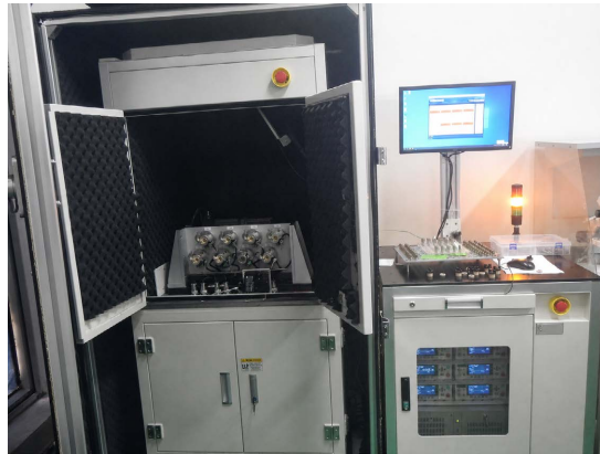
Figure 8. Physical diagram of the reliable foreign matter detection system based on vibration-current coupling.
