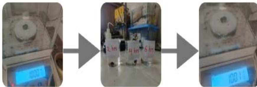
Figure 5. Water absorption test.
