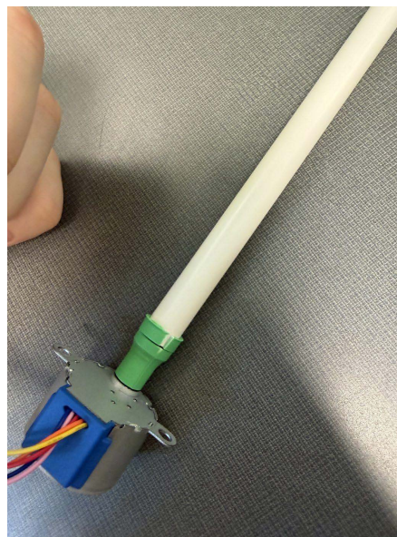
Figure 2. Physical prototype: coupler v3 installed on the 28BYJ-48 stepper output shaft and engaged to the host blinds tilt wand via the friction-fit sleeve.
