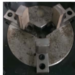
Figure 10. Design drawing and physical view of the universal clamping system.
