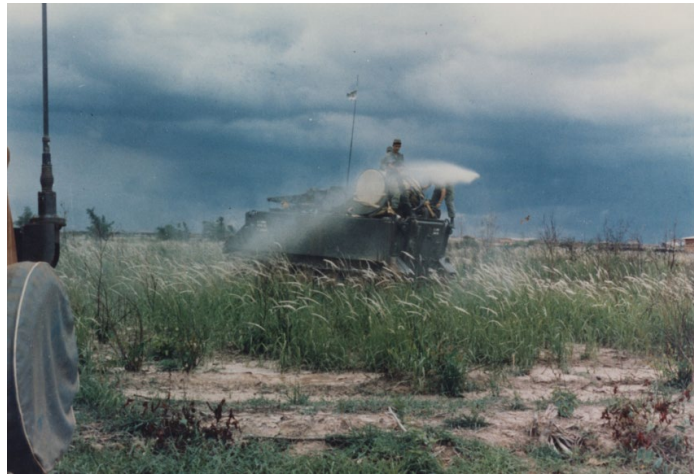
Figure 22. Tactical herbicides sprayed from a M113 Armored Tracked Personnel Carrier, Reprinted with the permission of the editor of the Open Journal of Soil Science.
