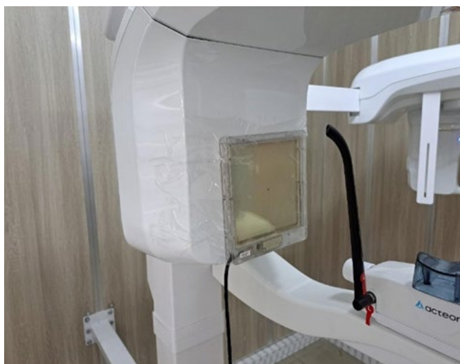
Figure 1. Attachment of the ionization chamber at the X-ray tube.
