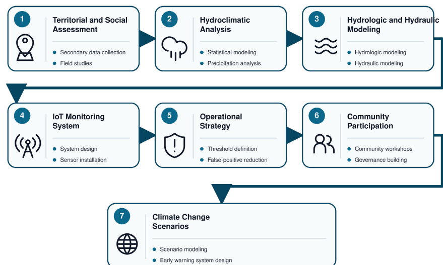
Figure 2. Integrated methodology for the Pacora River early warning system.
