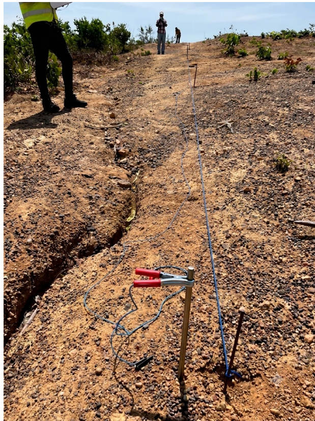
Figure 9. Field arrangement for Schlumberger dipole-dipole resistivity survey.
