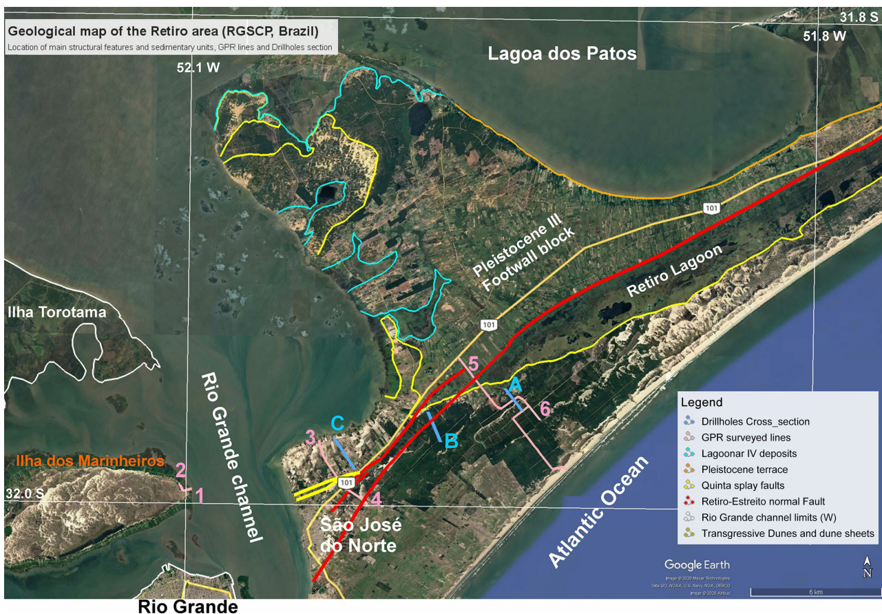
Figure 4. Detail geological map on both sides of Rio Grande channel, extending geological and sedimentary features previously discussed in [12]. The location of new GPR survey lines (1 to 6) and drillhole section (A, B, C) in the Retiro area is presented.
