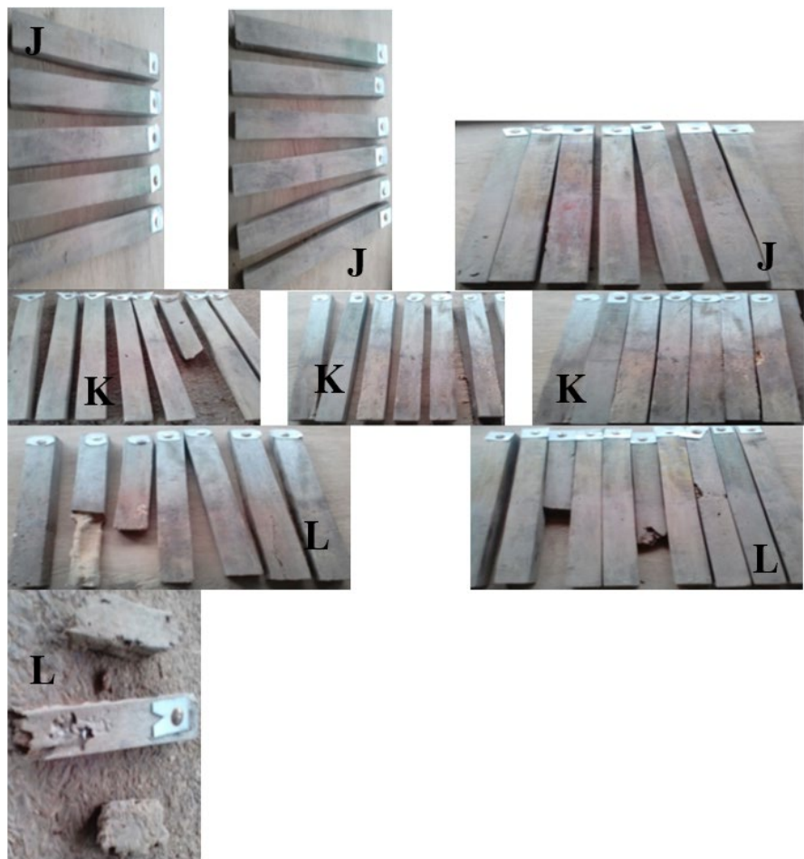
Figure 7. Termites' destruction on heartwood (J) sapwood (K), and control samples (L) after 12 months of field exposure (graveyard) test.
