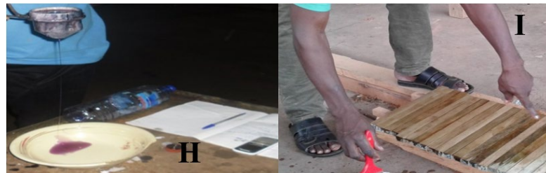
Figure 4. Sapwood (H) and Heartwood (I) air-dried after CCA-B impregnation.
