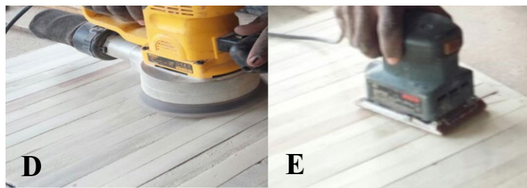
Figure 2. Sanding of samples using a disc sander (D) and an orbital sander (E).
