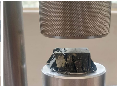
(b) Specimen between the platens
