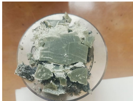
(c) Failed specimen on the lower platen
