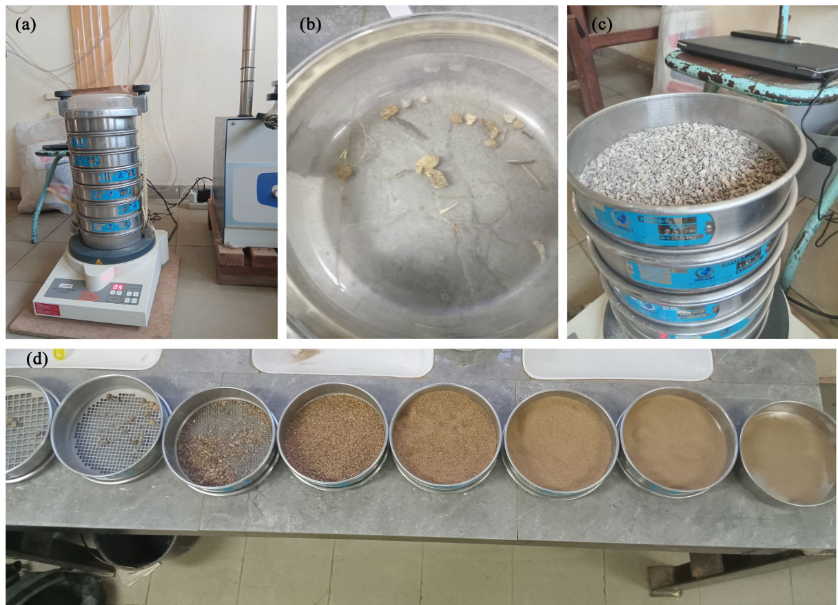
Figure 1. Sieving. (a) sieve column; (b) root and leaves of in river sand; (c) retained in 5mm sieve of M-sand; (d) sieving of sanaga (river) sand.
