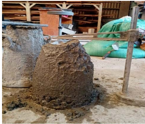
Figure 3. Concrete workability test setup.
