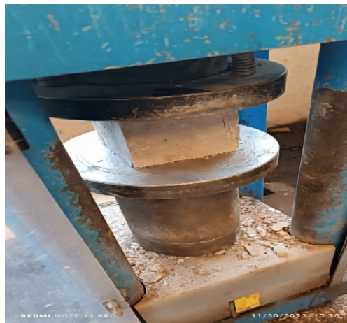
Figure 4. Experimental setup of compressive strength test.
