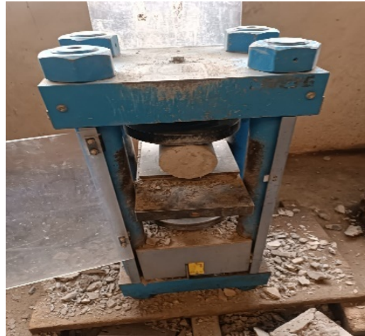
Figure 5. Experimental setup of tensile strength test.
