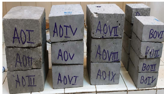
Figure 1. Pictures of specimens of rock blocks, types A (150 mm × 150 mm × 75 mm) and B (100 mm × 100 mm × 50).
