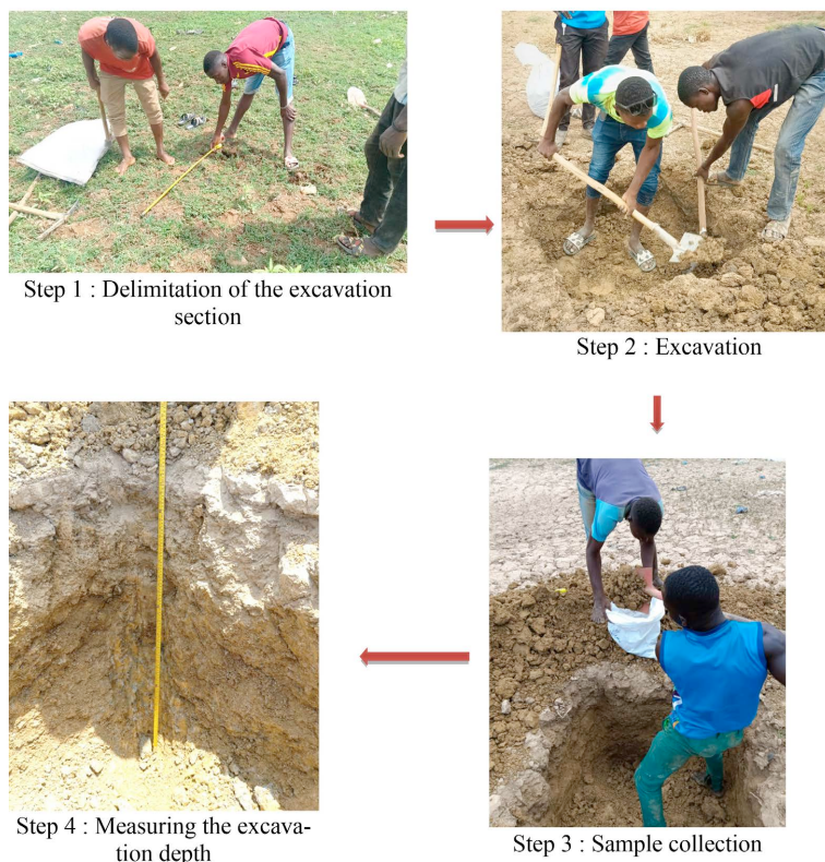
Figure 2. Process for collecting sediments from sites.
