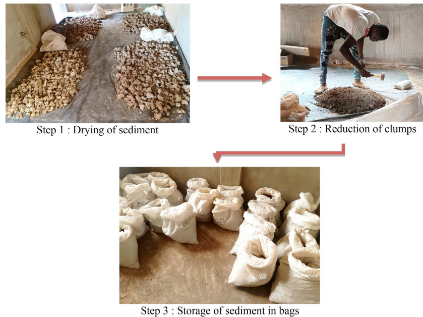
Figure 3. Preparation of sediment samples.
