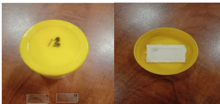
Figure 2. Closed and open view of dosimeter that consists of a cylindrical plastic bottle with detector fixed below the lid of the dosimeter.
