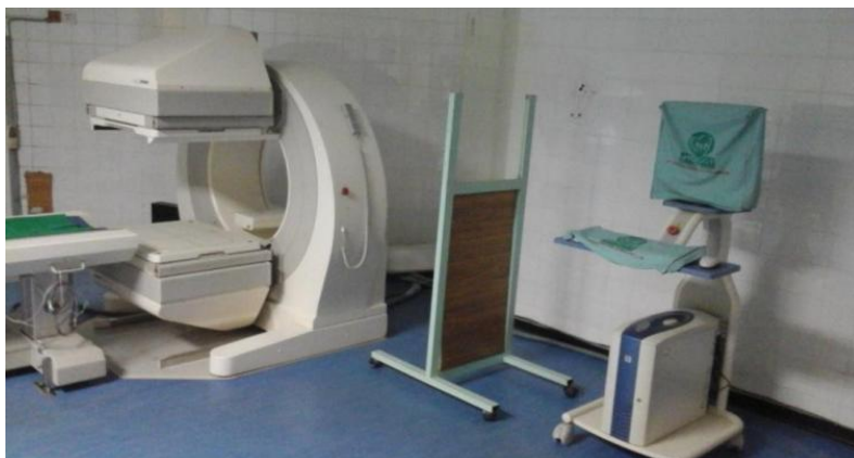
Figure 1. Dual-head SPECT Gamma camera of the nuclear medicine department of HOGIP and the acquisition console.
