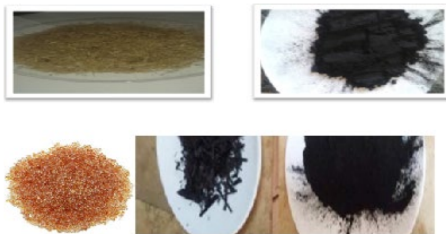
Figure 1. Images of activated carbon obtained from sugarcane bagasse before, after carbonization process, and natural zeolite.
