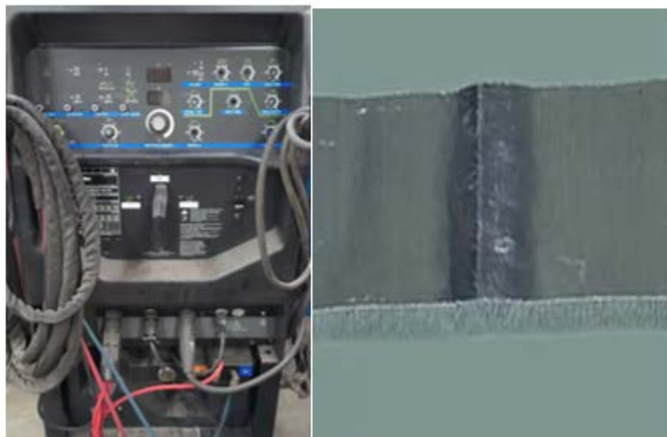
Figure 1. Miller Synchrowave 350 LX TIG welding machine/Butt Welded Joint.
