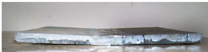
Plate 1. 10 mm mild steel plate sample with visible distortion.
