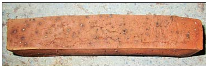
Figure 6. Visual appearance of specimens fired at 900°C for 45 minutes with 10% spent pot lining.
