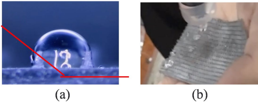
Figure 11. Photographs of water droplets on treated PDMS showing contact angles and hydrophobic/superhydrophobic performance testing.
