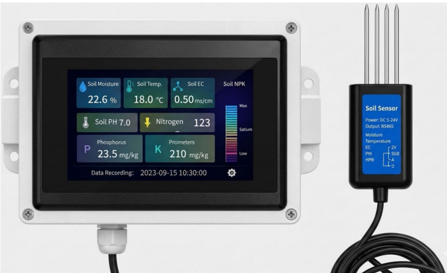
Figure 2. Soil controller and sensor (GHL Control Pad).
