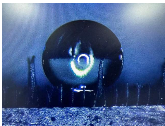
Figure 2. Measuring the water contact angle of the PDMS materials.
