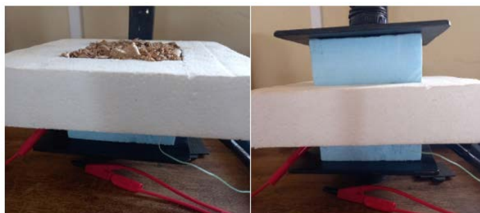
Figure 6. View of an asymmetric hot wire device for powdered or crushed fibre materials.
