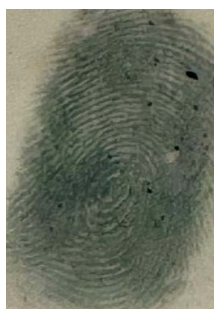
Figure 3. Fingermark on soft synthetic paper after its treatment with ninhydrin and visualized in daylight.
