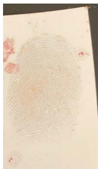
Figure 2. Fingermark on select synthetic paper after its treatment with ninhydrin and visualized in daylight.
