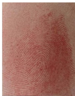
Figure 4. Fingermark on premium synthetic paper after application of Alizarin and visualized in daylight.
