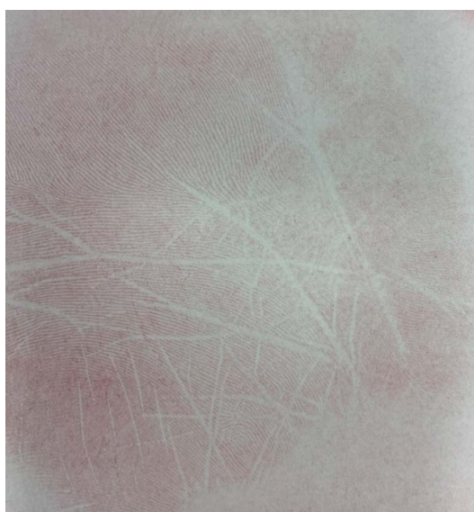
Figure 7. Palm mark on synthetic paper (polypropylene) after application of Alizarin and visualized in daylight.
