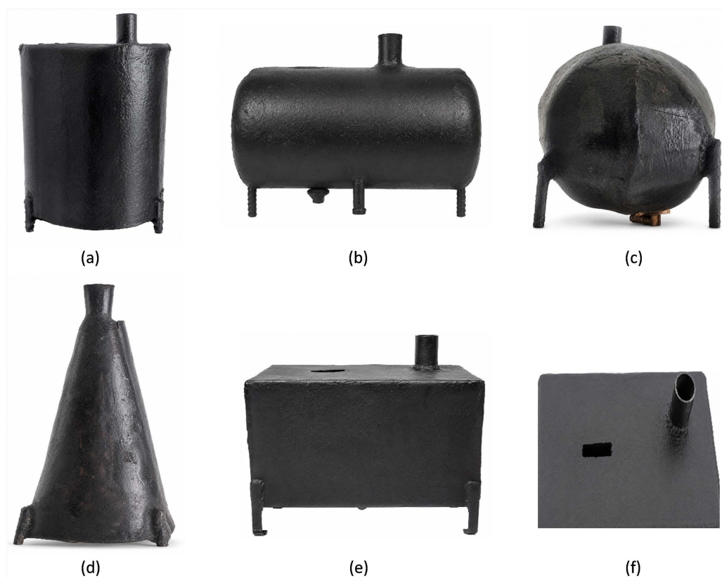
Figure 1. Pictures of fabricated storage vessels: (a) vertical cylindrical; (b) horizontal cylindrical; (c) spherical; (d) conical; (e) cuboidal; (f) upper section of cuboidal vessel.
