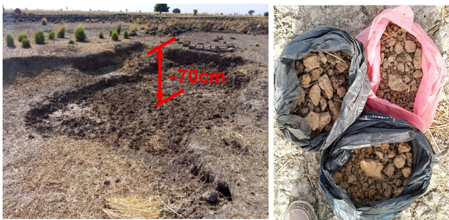
Figure 2. Artisanal clay extraction site in Zimado II: open excavation pit with visible clay-rich horizon and raw brick units in the background.
