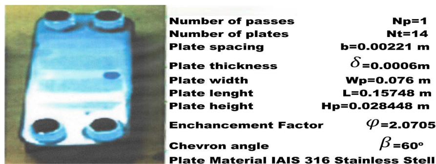
Figure 4. Chevron Plate Heat Exchanger—CPHE-1 [1].
