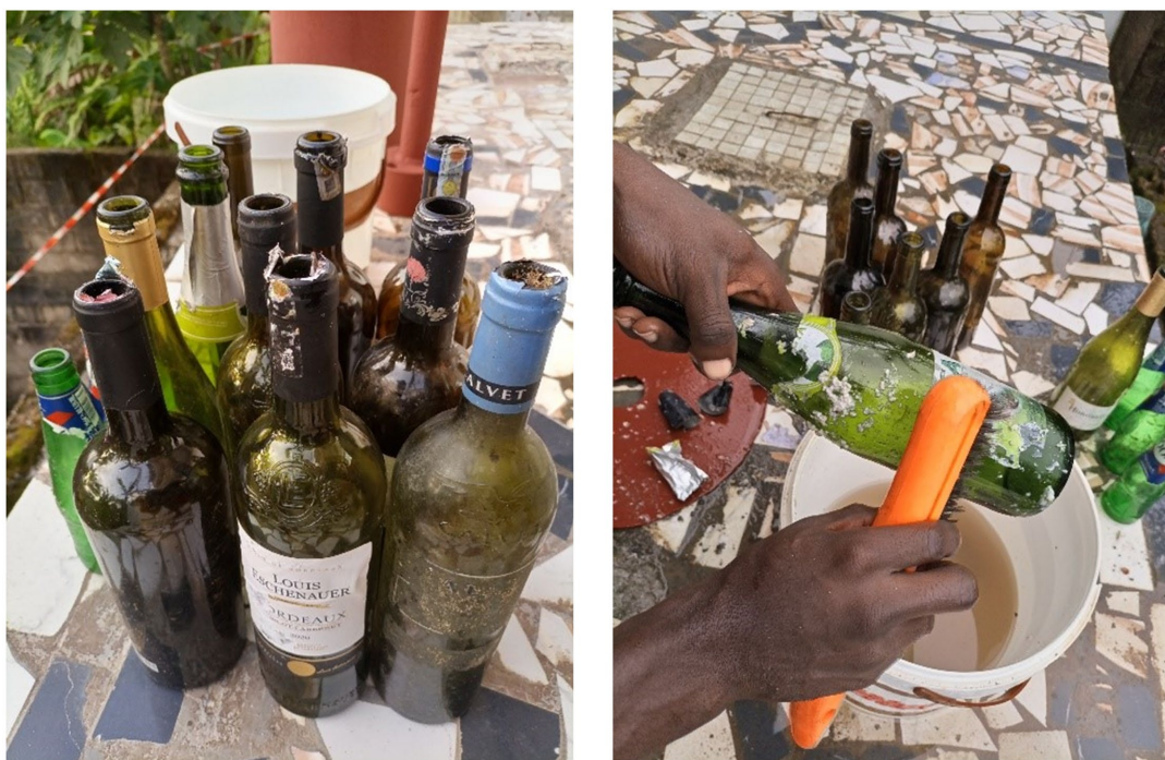
(a) Container glass collected from recycling facilities. (b) Cleaning and preparation stages prior to grinding.
