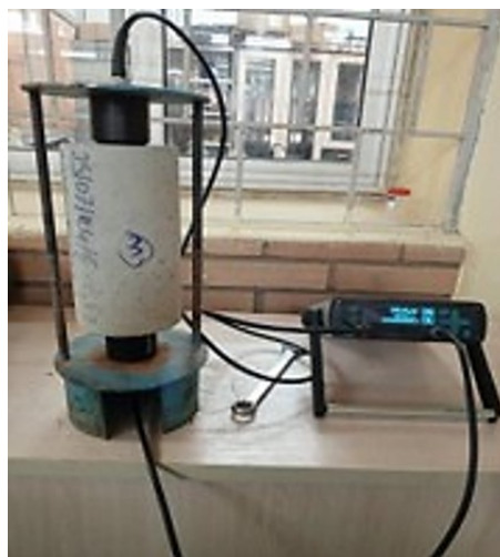
Figure 2. Experimental device of the ultrasonic pulse velocity test.
