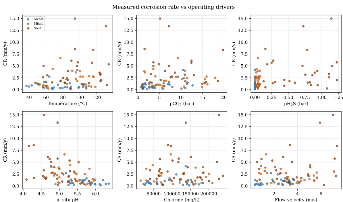
Figure 2. Measured corrosion rate versus operating drivers, coloured by service regime.
