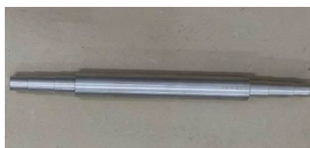
(a) Aluminum alloy shaft.
