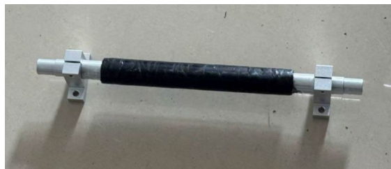
Figure 21. Fixing method of the shaft.
