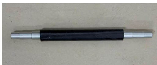
(b) Al/CFRP shaft.
