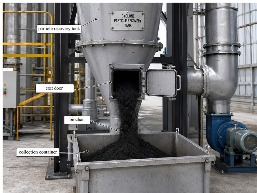
Figure 4. Emptying the cyclone particle recovery tank: charcoal powder (biochar) discharged through the coal powder exit door into a collection container.
