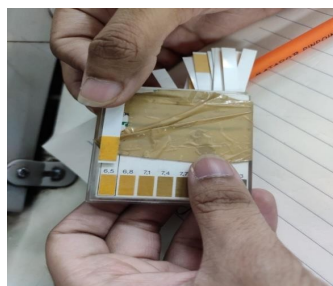
Figure 4. Neutral bath PH measurement.
