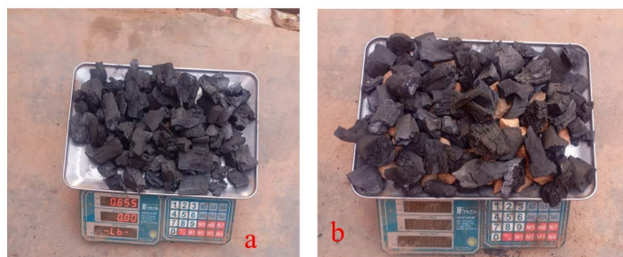
Figure 1. Fuels used: (a) coal combined with inert material; (b) coal alone.
