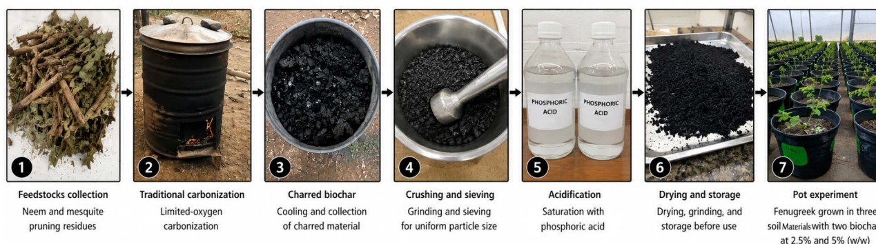
Figure 1. Workflow for producing acidified neem and mesquite biochars and applying them in the fenugreek pot experiment. The steps are feedstock collection, traditional limited-oxygen carbonization, recovery of the charred material, crushing and sieving, saturation with dilute phosphoric acid, drying and storage without washing, and application to three contrasting Sudanese dryland soil materials classified as Vertisol, Entisol, and Aridisol.
