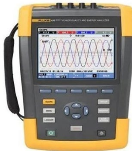
Figure 5. PQ data logger fluke 435.
