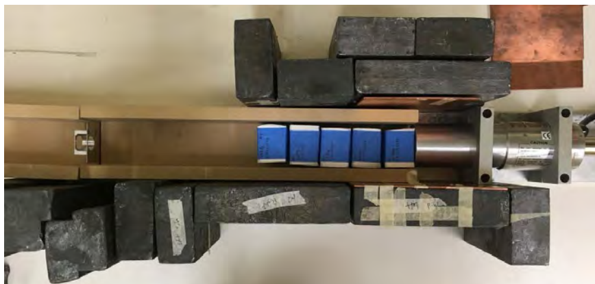
Figure 2. Top view of the Experimental Setup. Left to right: source holder, trough with organic blocks, HPGGe detector.
