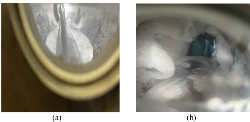
Figure 9. Images of CO 2 hydrate formation from water dropping at 0°C and 500 psi: (a) after 4 hours, (b) after 24 hours.
