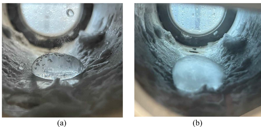
Figure 11. Images of CO 2 hydrate formation during water dropping at 3°C and 500 psi (near the equilibrium point): (a) a water pocket stayed at the bottom of CO 2 liquid at the beginning, (b) a hydrate-shelled water pocket stayed at the bottom side of the reactor after 12 hours.
