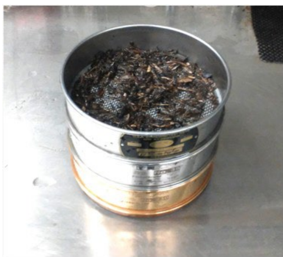
Figure 3. Stacked sieves were used to produce control sediments from commercial topsoil, and to process site soil with significant amounts of large organic matter.
