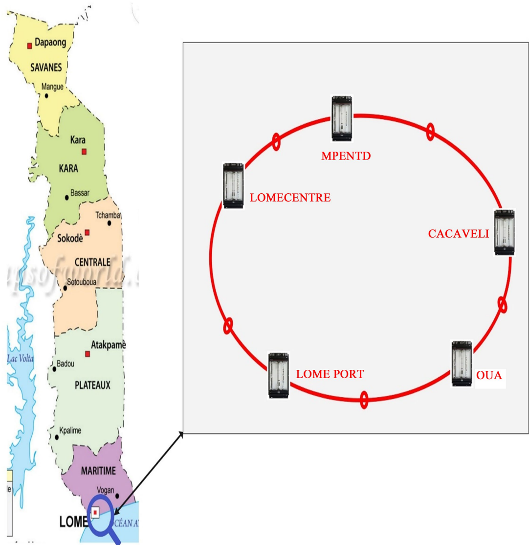
Figure 1. 30 km Backbone Network architecture.
