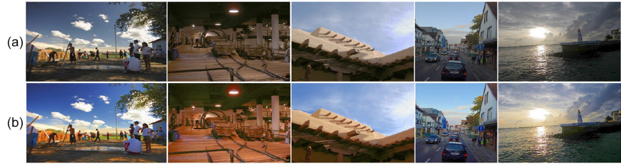
Figure 2. (a) Original low-light images; (b) After applying PCGF.
