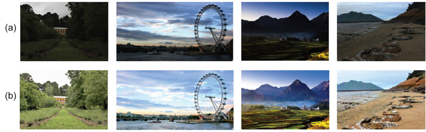
Figure 7. Physical Illumination Modeling (a) Original Images and (b) ALSM results with T = 6 , where T denotes the number of pyramid decomposition levels used in the multi-scale fusion step.
