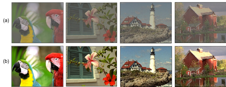
Figure 6. Histogram equalization results, (a) Original images and (b) AHE-processed images.
