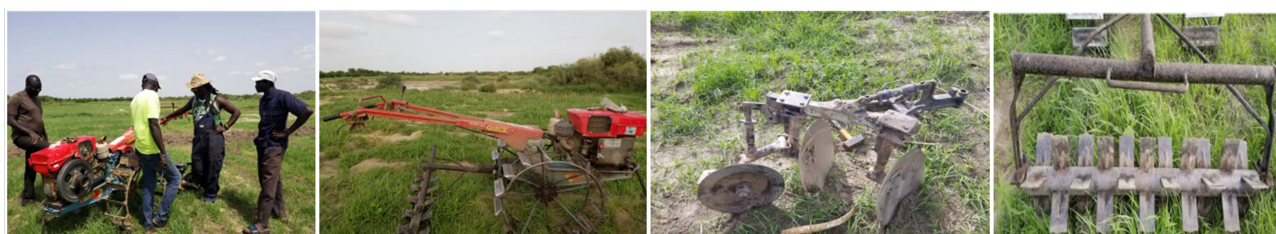
Photo 1. Motorized tiller, or walking tractor, equipped with a disc plough. The accessories included an offset disc harrow for land preparation and a puddling attachment for soil leveling and puddling operations.
