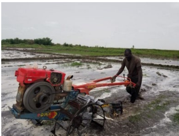
Photo 2. Walking tractor operation with the puddling chain.
