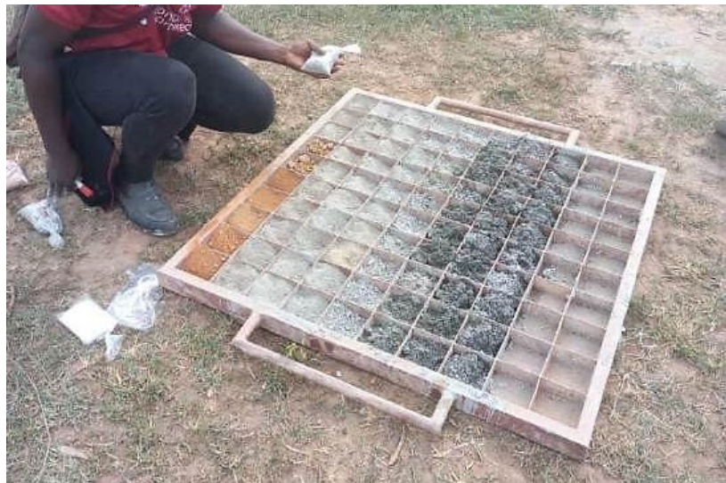
Figure 4. Boxing of crushed samples collected at one-meter intervals in the Dikodougou area, Northern Côte d'Ivoire.
