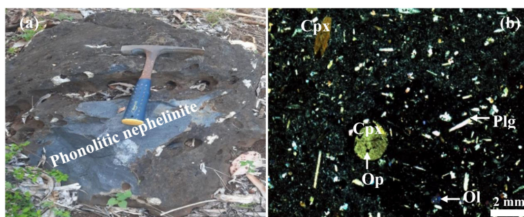
Figure 7. (a) (b) Macroscopic and microscopic characteristics of a phonolitic nephelinite showing rare clinopyroxene (Cpx) microphenocrysts within a very abundant groundmass rich in plagioclase (Plg), olivine (Ol), and opaque mineral (Op) microlites.
