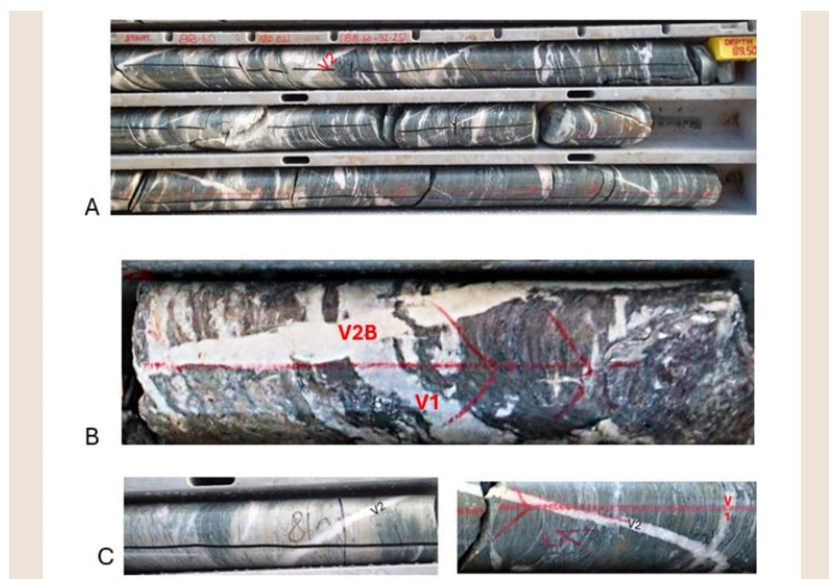
Figure 8. Quartz vein V2 generations at Aburna gold district. V2 veins at Hill 52. (A) V2 veins in a chlorite, carbonate, and epidote schists ABD011, 89 m. (B) V2B veins of calcite crosscutting quartz-carbonate-pyrite V1 vein in a fault zone, ABD014, 185 - 188 m. (C) Left, N-trending vertical V2 vein crosscutting S1 in an anticlockwise sense, Right, E-W-trending v2 veins crosscutting S1 in a clockwise direction, ABD011, 81 and 84 m.
