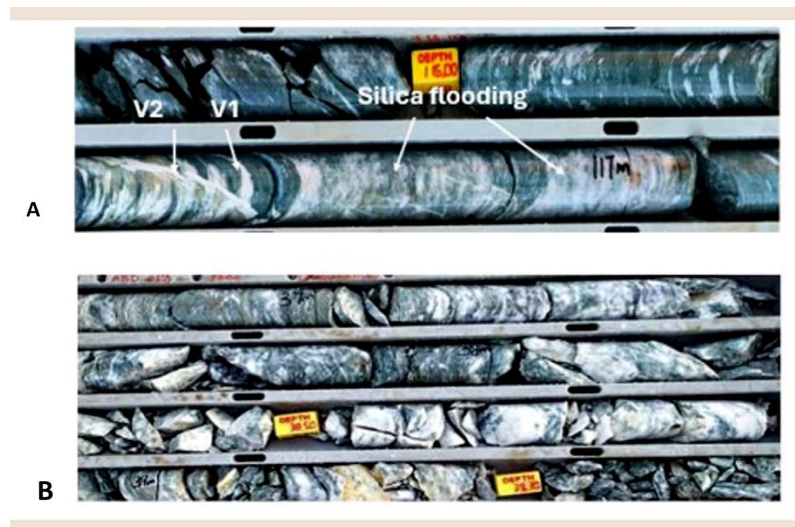
Figure 9. Core drill photographs of silica flooding. (A) ABD012, 117 m; (B) Silica flooding within a major ductile-brittle fault ABD013 from 36 to 41 m.
