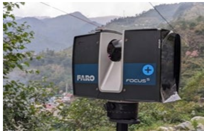
Figure 1. FARO S350+ (Scanner).
