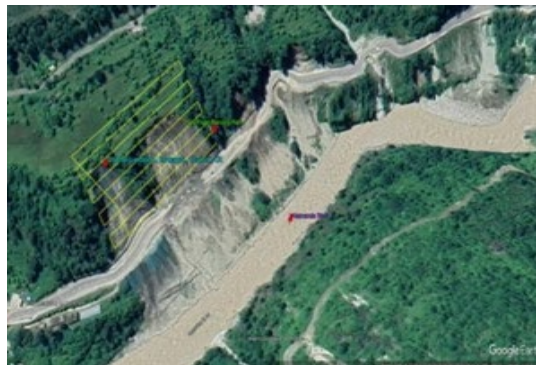
Figure 9. Flight planning of UAV.
