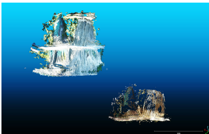
Figure 11. Fusion of point cloud DATA (UAV-2022 and TLS-2022).
