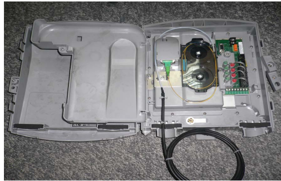
Figure 3. Optical Network Terminal (ONT).
